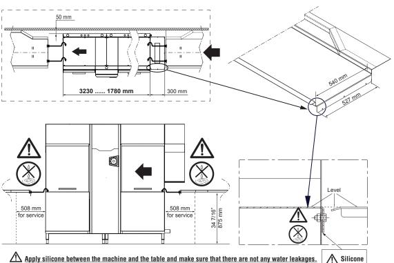
Apply silicone between the machine and the table and make sure that there are not any water leakages.
